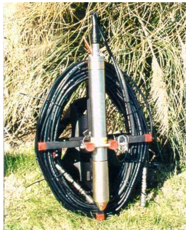
DHS-5500 Downhole Source
