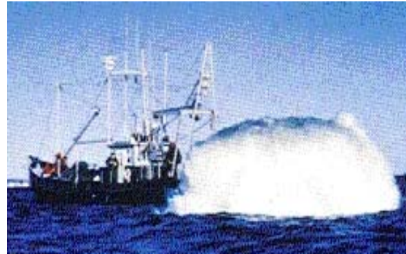
▲ Bubble Venting from a 9000 in 3 Air Gun at 10 m. depth
